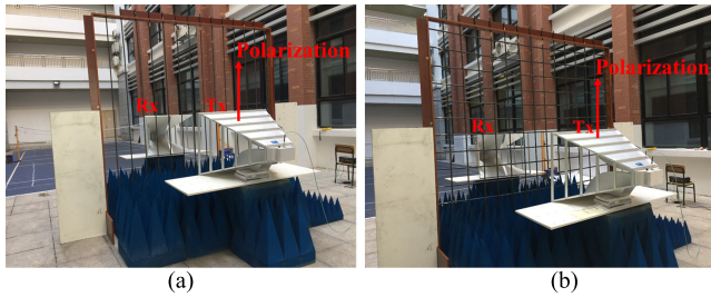
Fig. 6. Laboratory experiments on (a) 1-D rebar array and (b) 2-D rebar net. The vertical and horizontal bars are tied together at the crossings.
